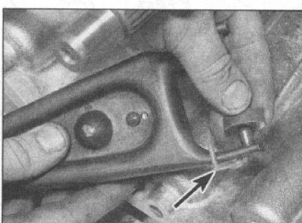
3.15b . . . and recover the release bearing guide slippers. Note release bearing securing clip (arrowed)
