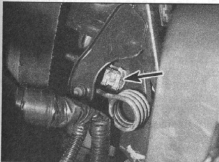
6.5 Master cylinder pushrod-to-clutch pedal clevis pin spring clip (arrowed)
